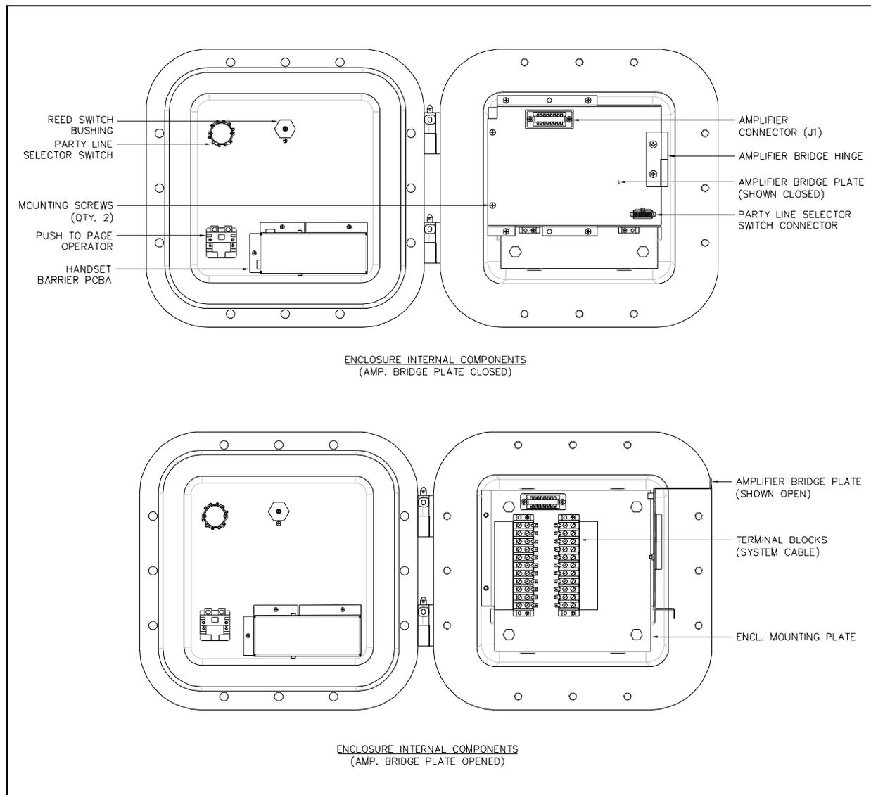
Figure 3. Model 7085-001-EX-F07044 Amplifier Enclosure - Interior View
