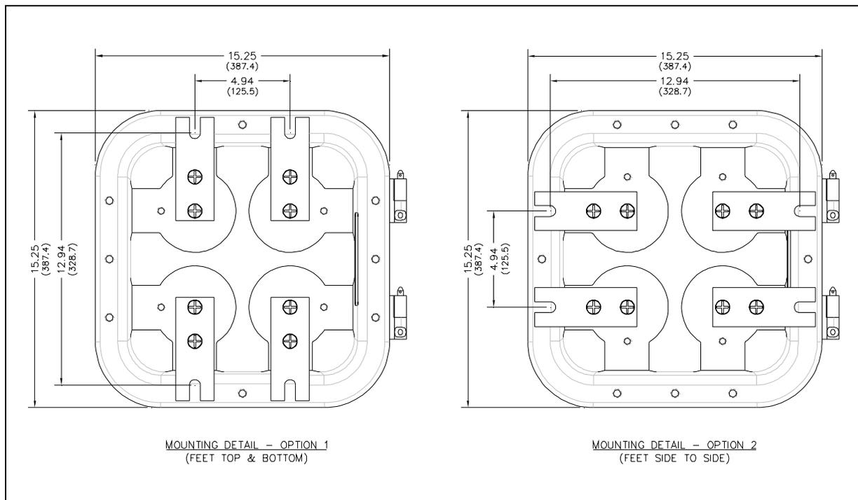
Figure 4. Model 7085-001-EX-F07044 Enclosure Mounting Details
