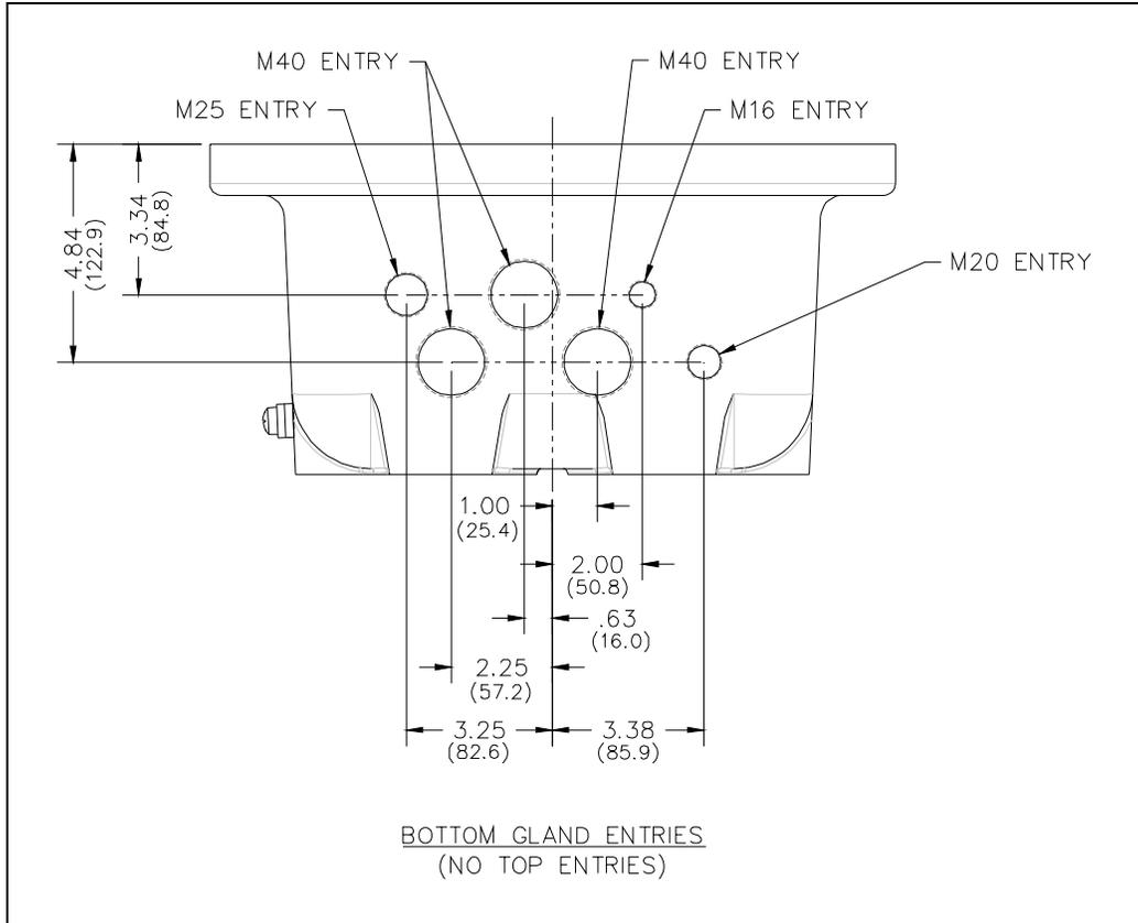
Figure 5. Model 7085-001-EX-F07044 Cable Gland Entries
